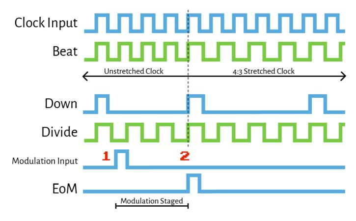
Notice that after the modulation, the *beat* output matches the *divide* output. Also, the time between two output clocks on the *down* output stretches by a factor of 4/3, reflecting the change in tempo. Finally, notice that the input clock and the *beat* output are no longer in sync, and now shift in and out of phase.
